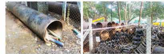
To the left is an image of cast iron pipes which have been partly corroded, abandoned beside the BWS&B building at Krishna Rao park to be picked up by dealers of scrap metal. This design proposes treating the pipes for corrosion removal and treatment and powder coating the pipes red for reuse.
